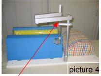
For an improved ultrasonic sensor movement a Sonoguide can be used optionally.
